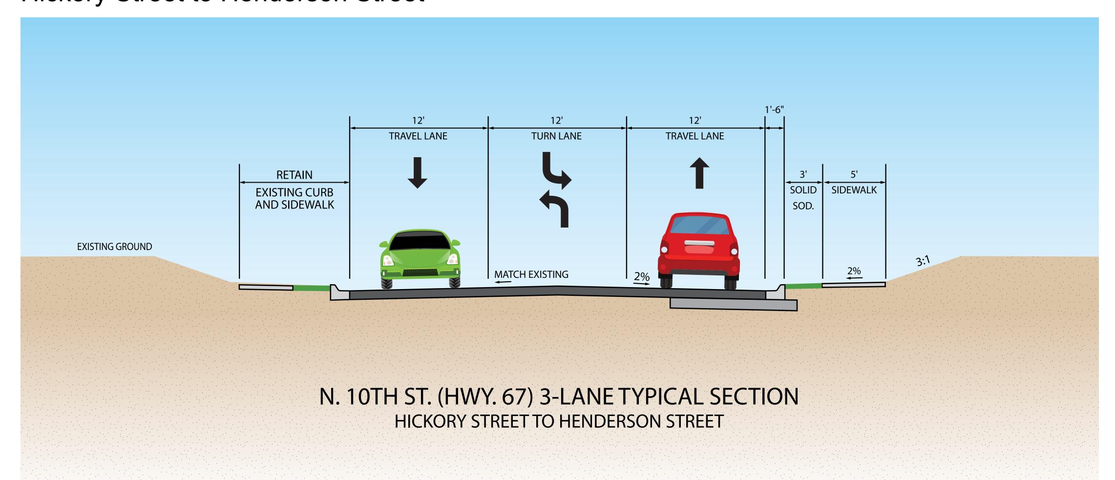
The typical section for North 10th Street between Hickory and Henderson Street also consists of two 12-foot-wide travel lanes and a middle 12-foot-wide turn lane with curb and gutter and sidewalks. The primary difference with the one above is the existing curb and sidewalk on the west side of the street will be retained.
