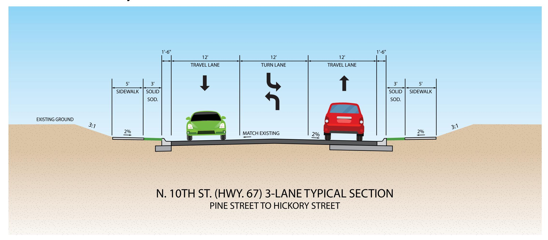
The typical section for North 10th Street between Pine Street and one block north to Hickory consists of two 12-foot-wide travel lanes and a middle 12-foot-wide turn lane, with curb and gutter, 5-foot-wide sidewalks, and sod between the roadway and sidewalks.
